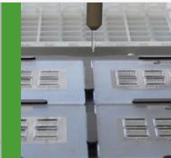
iTWO-400 for flexible deck configuration with MTPs and targets next to each other
