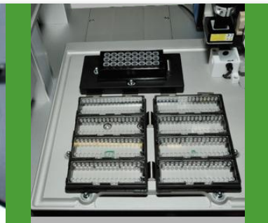
instrumentTWO equipped with 100 \mu L source vials and 8 Lab-on-a-Chips microfluidics
