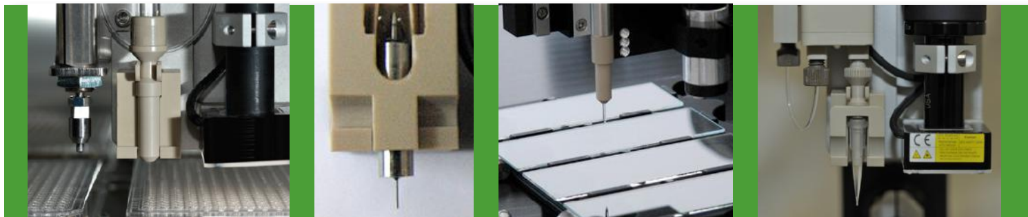
instrumentONE equipped with PDMD, piercer for sealed plates (left) and head camera (right)
